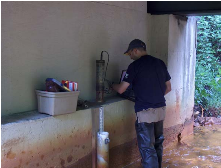
Figure 3. Ben Mack downloading data from a Eureka sonde on lower Greens Run.
