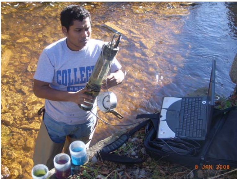
Figure 4. Joseph Kamalesh calibrating a Eureka sonde on the South Fork of Greens Run.
