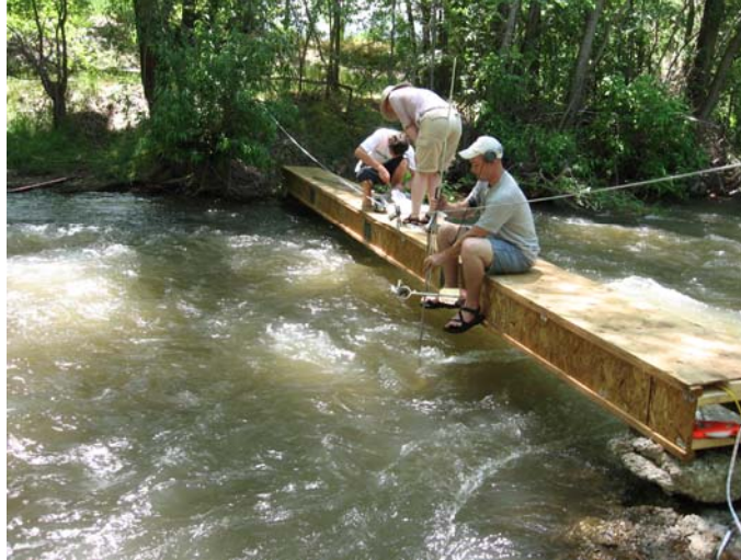
Figure 6. Students taking discharge measurements and bedload samples from a footbridge.
