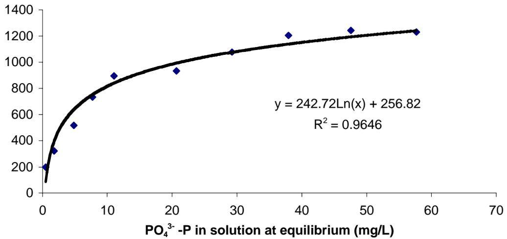
Figure 4. Results of sorption isotherm conducted at 22°C.
