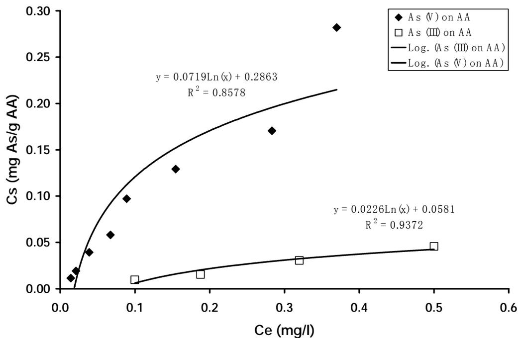
**Figure 3.** Adsorption isotherms of As(V) and As(III) on activated aluminum.
