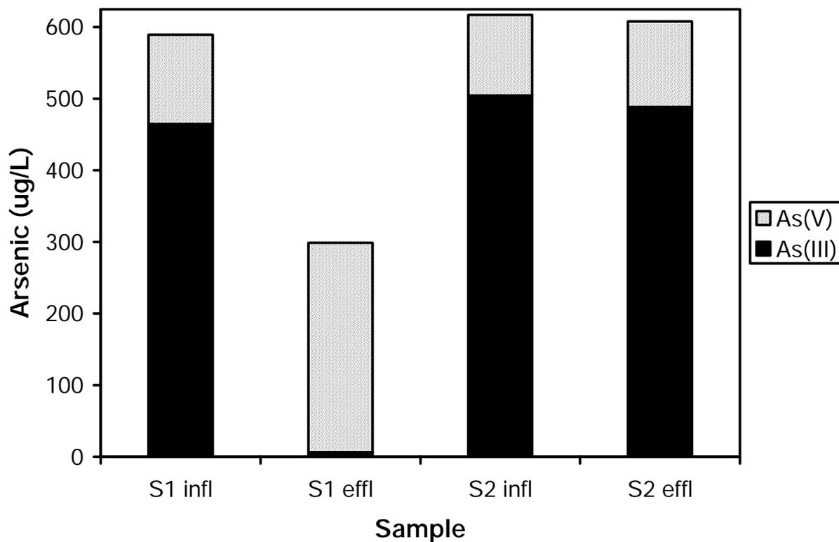
**Figure 5.** Speciation of arsenic in influent and effluent samples of activated alumina packed columns containing  $\text{NO}_3^-$  (S1) or lacking  $\text{NO}_3^-$  (S2).
