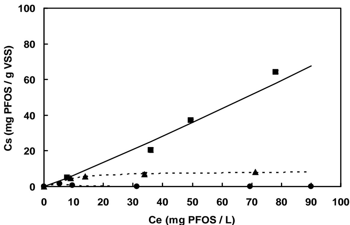
**Fig. 8.** Adsorption isotherms of PFOS onto wastewater treatment sludge. Legend: (■) anaerobic granular sludge, (▲) anaerobic digested sludge (●) activated sludge; (dashed line) experimental data fit to Langmuir model; (solid line) experimental data fit to Freundlich model.
