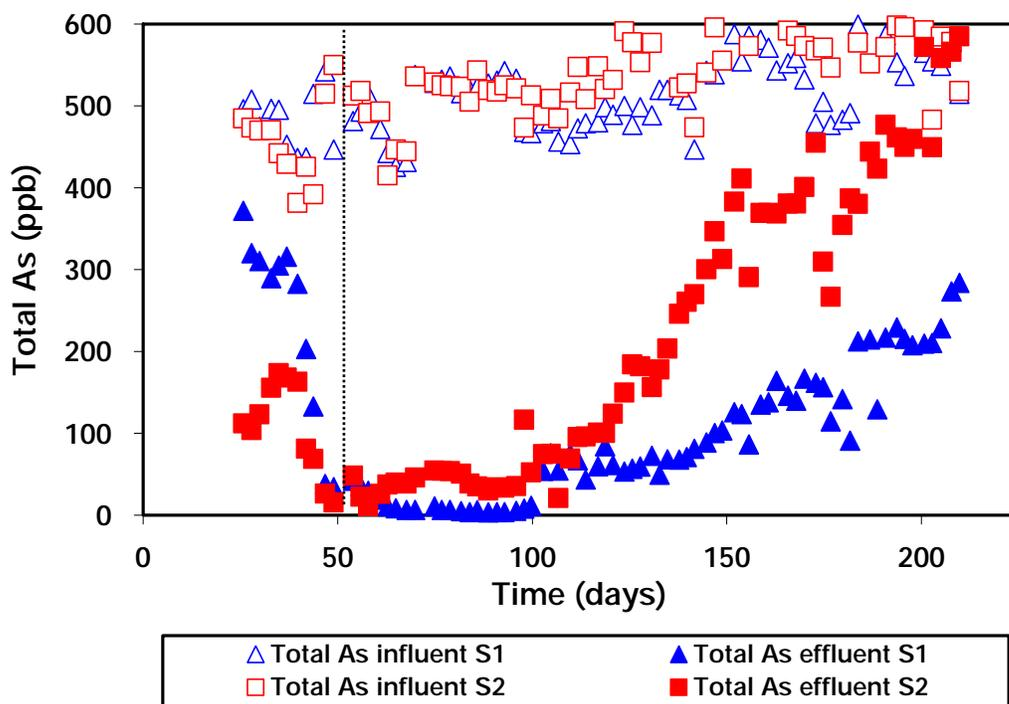
**Figure 4.** Influent and Effluent concentrations of total arsenic entering activated alumina packed bed columns S1 (with  $\text{NO}_3^-$ ) and S2 (without  $\text{NO}_3^-$ ). The vertical line on day 50 indicates the time point, after which the pH was controlled around 7.5, prior to day 50 the pH was alkaline (8 to 10).
