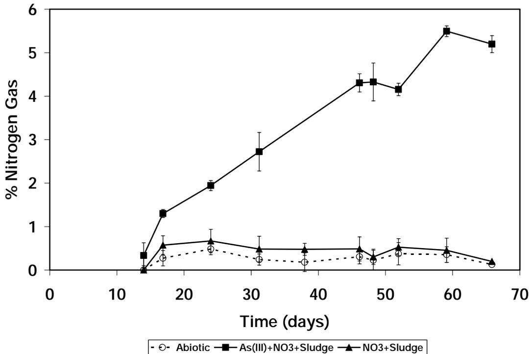
**Figure 2.** Formation of  $N_2$  gas from the oxidation of As(III) linked to denitrification. Bottles were incubated with 3.5 mM As(III) with 0.6 g volatile suspended solids/L
