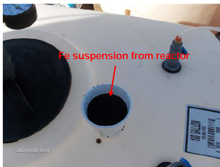
Figure 1. A picture of the CMC-stabilized Fe-Pd particles (Fe = 1 g/L) taken from the reactor 5 min after preparation. The dark color indicates the presence of ZVI nanoparticles which are fully dispersed in the water solution.
