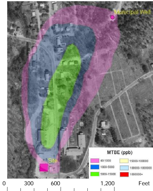
Figure 1: Currently known extend of the Pascoag MTBE plume in the bedrock aquifer.
