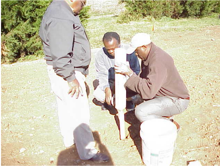
Figure I. Lysimeters being installed in the poultry pellet amended plot by William Hare and James Allen.
