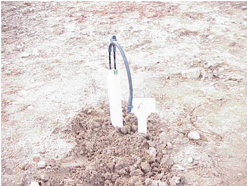
Figure II. Lysimeter in place at a depth of 18 inches.
