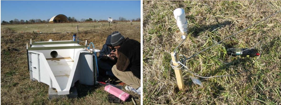
Figure 1. Instrumented hillslope with surface and subsurface sensors (detailed view on the right), H-flume, rain gage, and shallow wells at the Sand Mountain Research and Extension Center, Crossville, Dekalb County, Alabama.
