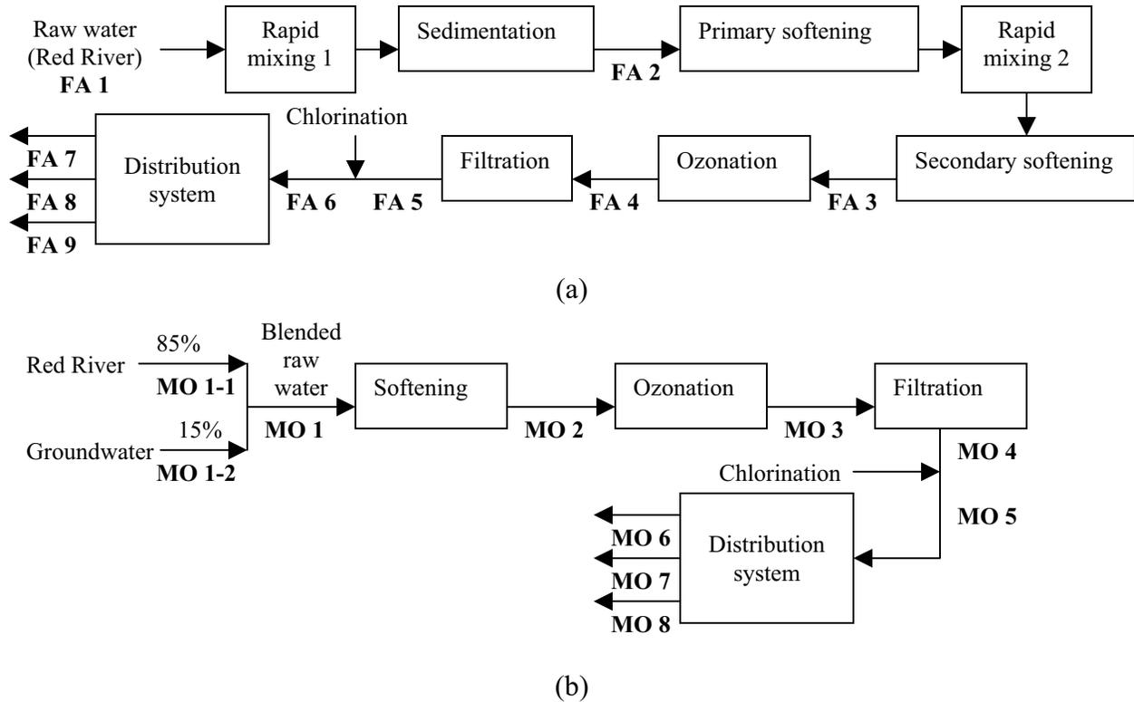
Figure 1 Simplified schematic diagrams for (a) the Fargo Water Treatment Plant and (b) the Moorhead Water Treatment Plant.
