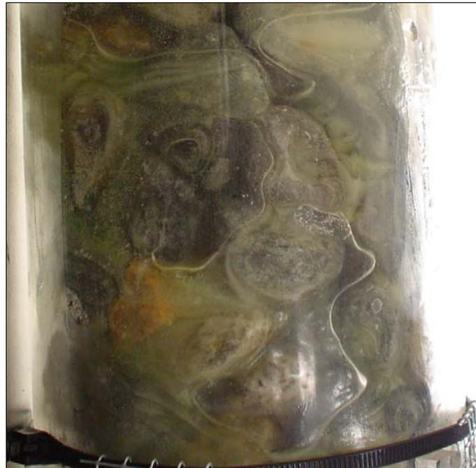
Figure 3: Large volumes of entrapped air form because of dead end pores
