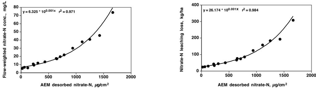
Fig 2. Relationship between soil nitrate-N desorbed from anion exchange membranes (AEMs) and flow-weighted nitrate-N concentrations and leaching losses of percolate collected from Kentucky bluegrass grown in soil columns. Each data point represents the mean of four replications.
