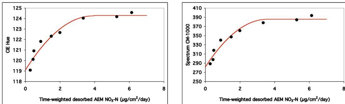
Fig 1. Relationship between soil nitrate-N desorbed from anion exchange membranes (AEMs) and CIE hue angle (greenness) and relative chlorophyll (Spectrum units) collected from a Kentucky bluegrass-perennial ryegrass-creeping red fescue lawn. Each data point represents the mean of four replications.
