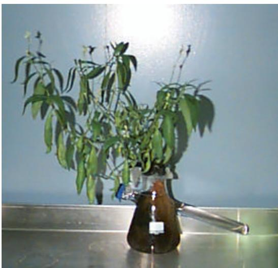
Figure 2. Experimental system used to quantify  $\text{O}_2$  released from wetland plant roots (*P. pennsylvanicum* shown).
