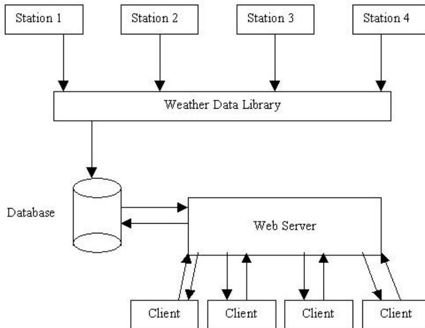
Figure 1. General structure of the system with a basic three-tier architecture associated with most Internet applications.
