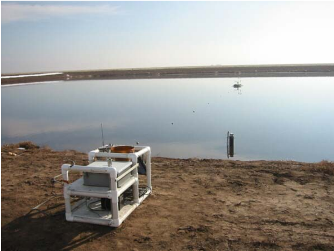
Figure 3. Using the bulk transfer approach of Ham (1999, 2002) to measure seepage from a swine waste lagoon.
