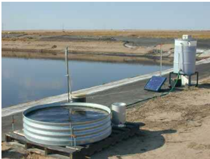
Figure 2. Photograph of the evaporation pan system in the field.
