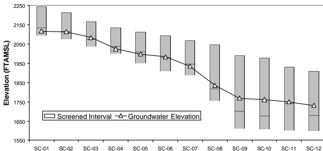
**Figure 3.** Santa Cruz monitoring well elevations (above mean sea level), screen intervals, and water table elevation. Tops of the lightly shaded portions of each bar represent the local elevation of land surface at the SC-series wells.
