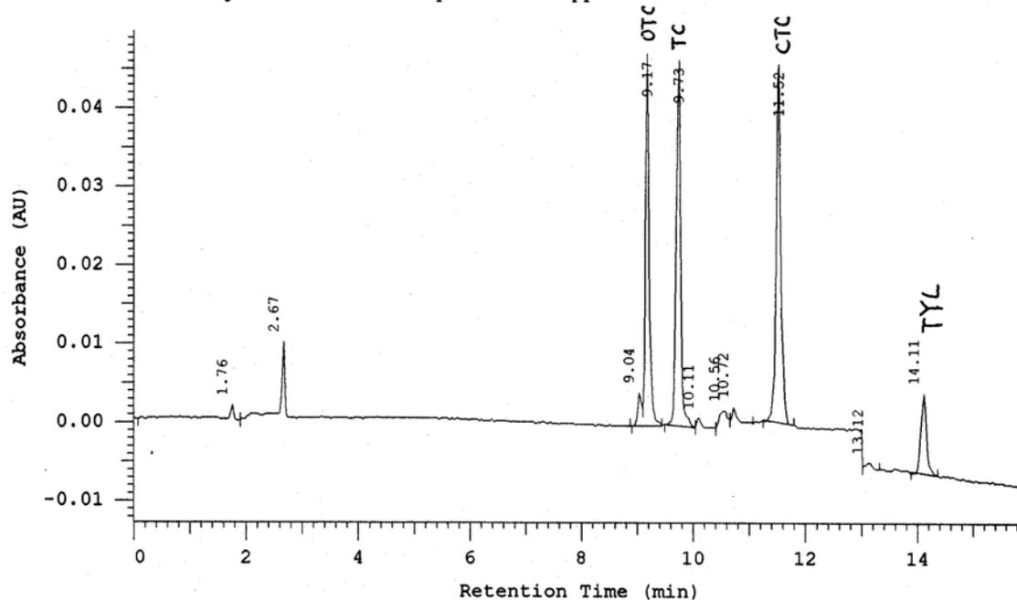
Clearly, with the setting we developed, these antibiotics are well separated. We calculated the recoveries tabulated in the following Tables. The recoveries are generally within the range of 50-120%. We also found that the water sample collected near the animal farm contains tetracycline and tylosin but not oxytetracycline and chlorotetracycline. These results will be highly useful in the further survey of antibiotics in Northwest Arkansas surface waters.
