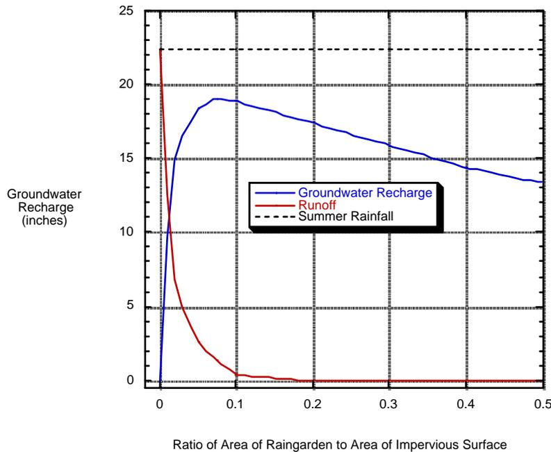
Figure 4 Results of the model of an impervious surface draining into a raingarden.
