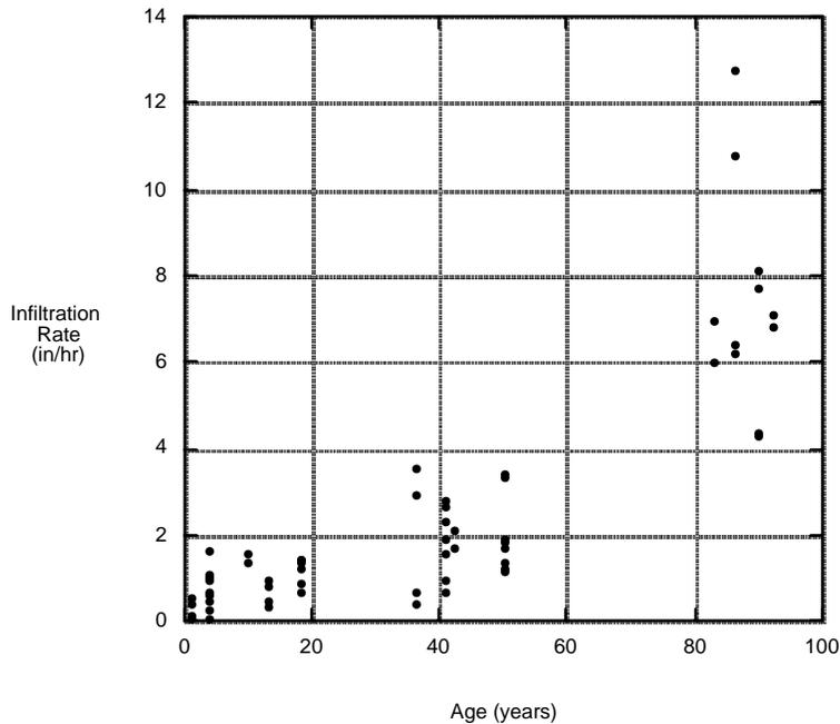
Figure 2. Unit-area infiltration rate vs. age of developed area.
