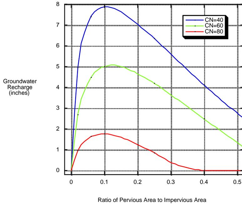
Figure 3. Results of the model of an impervious surface draining onto a pervious surface.
