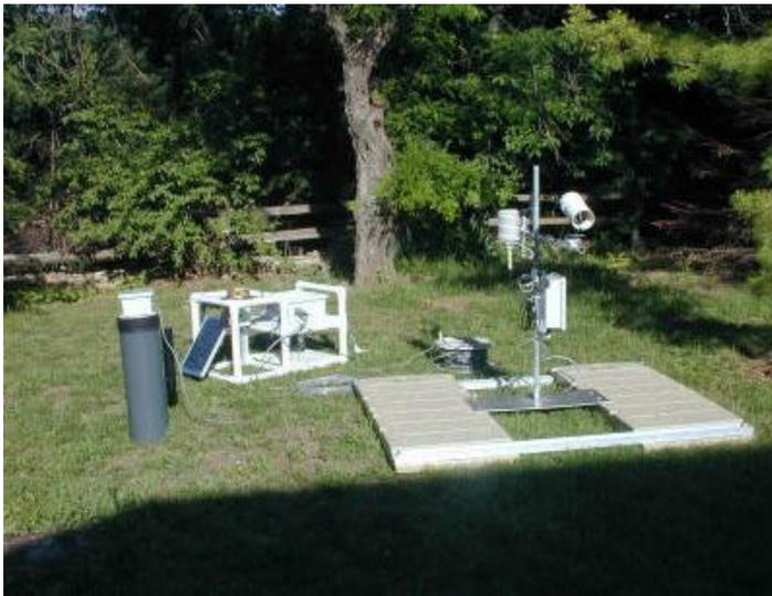
Figure 3. Photograph of the equipment required to implement the bulk transfer approach of Ham (1999).
