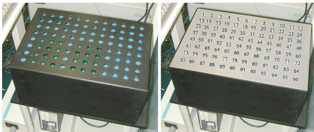
Fig. 33.5. Heated block used for carbonate-acid reactions at the University of Rochester. Right shows vial numbers used by the IRMS. Courtesy P. Higgins, University of Rochester, Rochester, NY.
