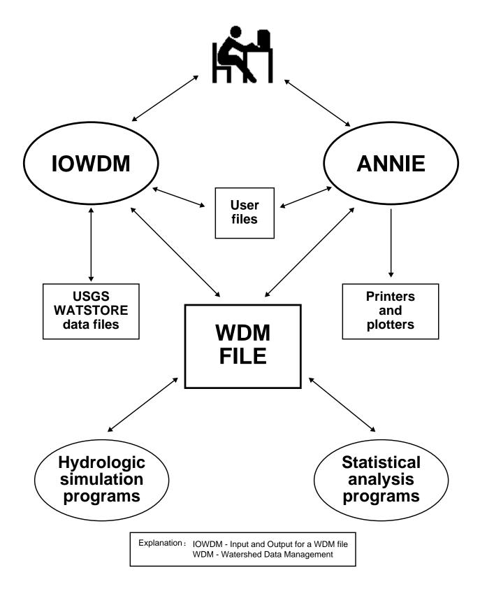
Figure 1. ANNIE and WDM system interactions and functions.
