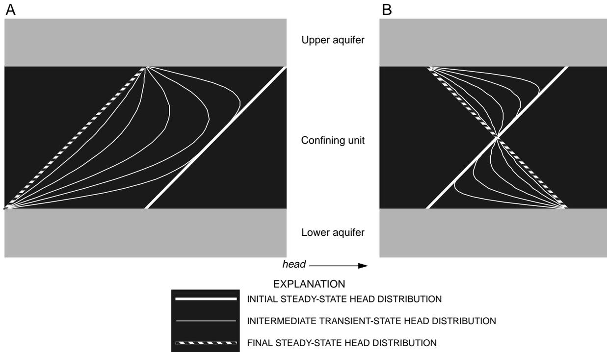
**Figure 2.** Distributions of head in a confining unit before and after head changes in overlying and underlying aquifers. Assumed initial conditions are steady-state flow from upper to lower aquifer. *A*, Head decreases equally in upper and lower aquifers. *B*, Head decreases in upper aquifer and increases in lower aquifer. Adapted from Trescott and others (1976).
