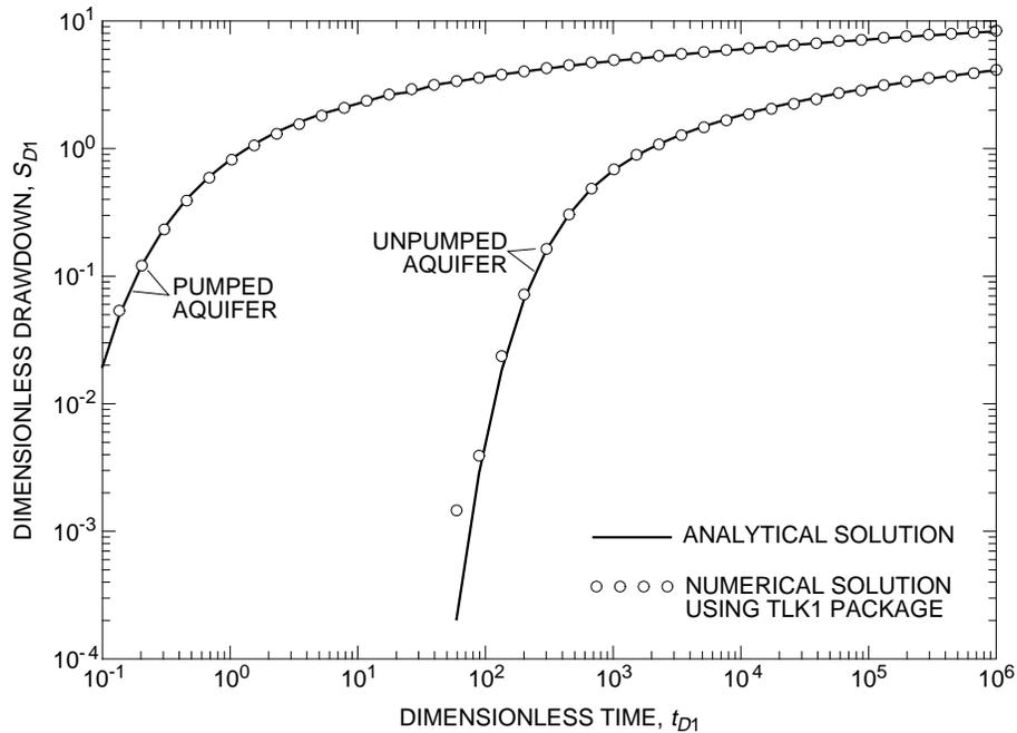
**Figure 10.** Results of problem 2 using the TLK1 Package to simulate the confining unit.
