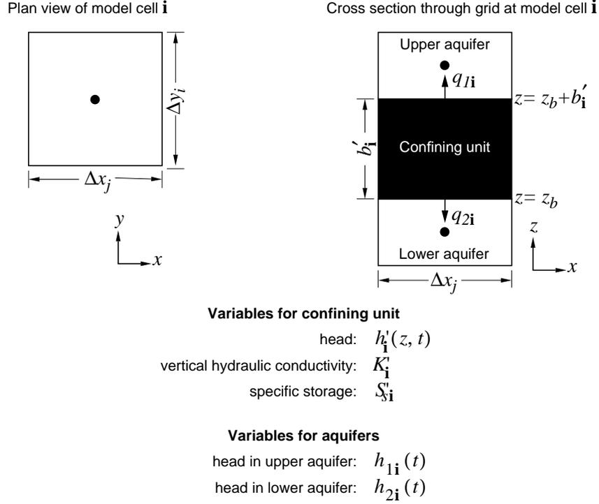
**Figure 3.** Variables used in development of transient-leakage equations for model cell  $i$ .
