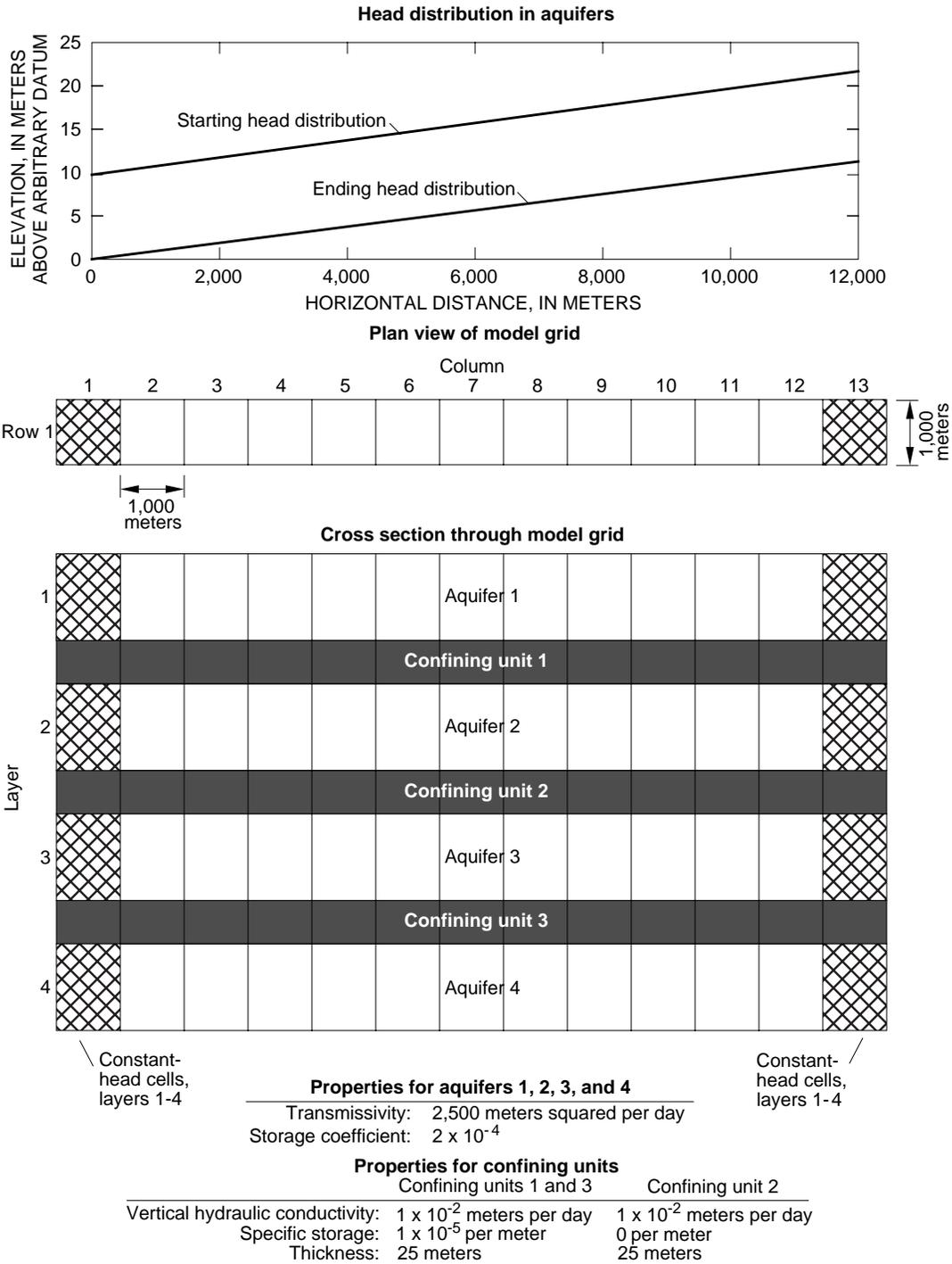
**Figure 7.** Head distribution, model grid, boundary conditions, aquifer properties, and confining-unit properties for problem 1.
