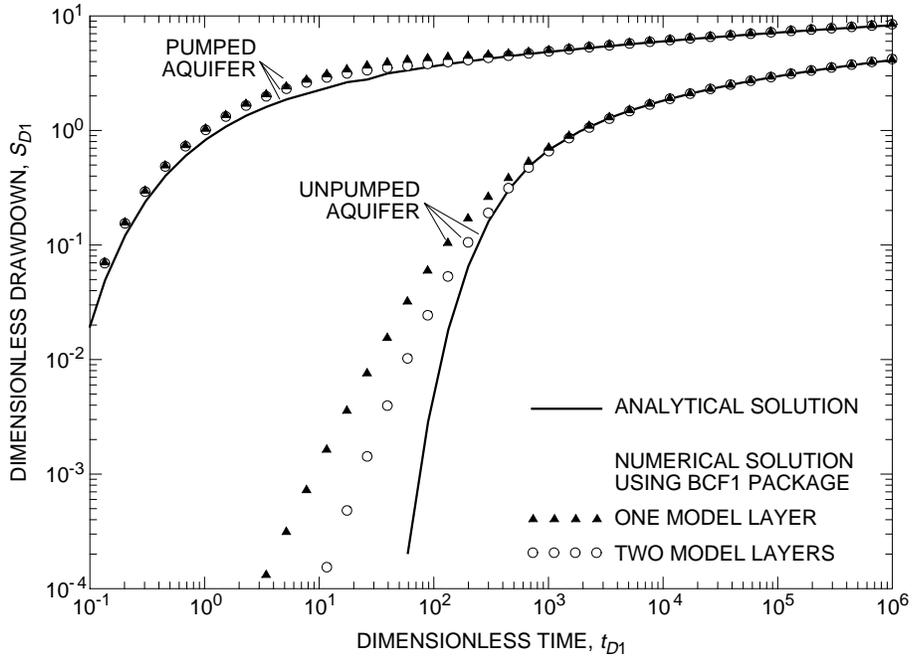
**Figure 11.** Results of problem 2 using the BCF1 Package with one and two model layers to simulate the confining unit.
