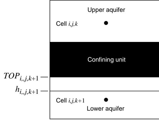
**Figure 6.** Situation in which a correction is needed to limit the downward flow into cell  $i,j,k+1$ . (From McDonald and Harbaugh, 1988).
