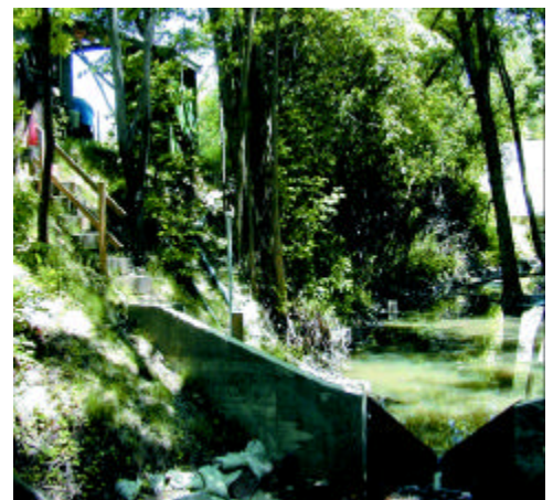
Figure 3. The USGS Englesby Brook monitoring station and site. The v-notch weir is in the lower right of the picture, and the stream-gaging station is on top of the high river bank to the left.
