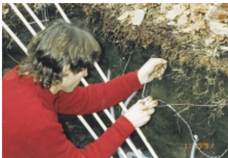
Figure 4. Hydrologist installing soil-temperature probes in a soil pit at Sleepers River.
