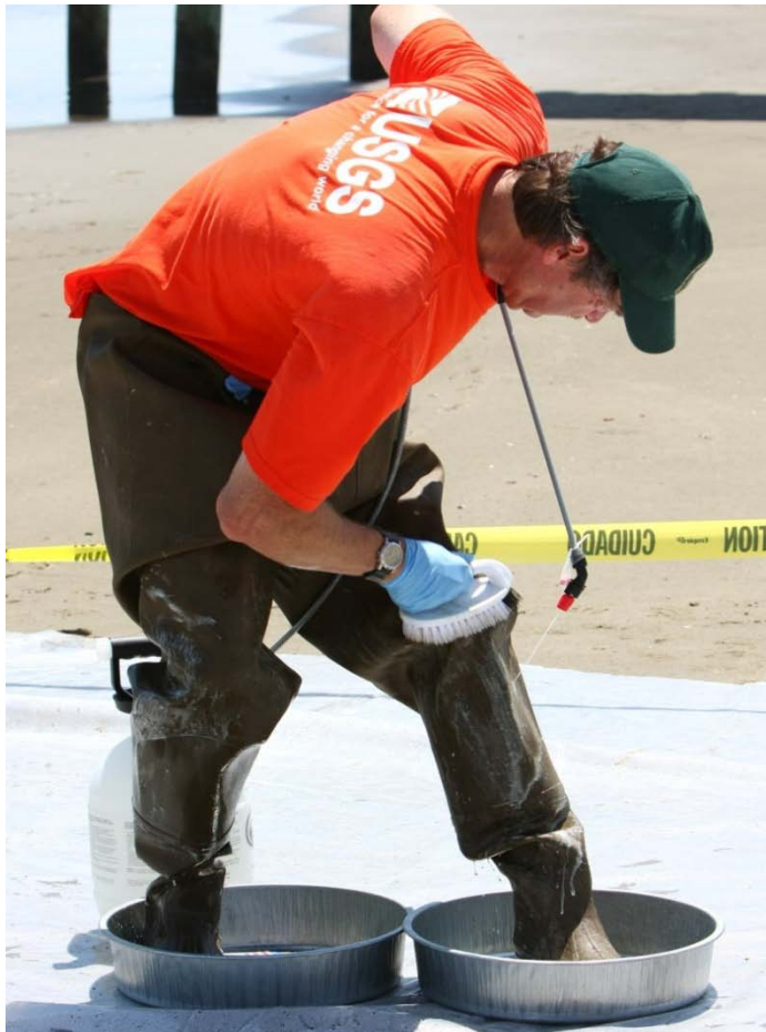
Figure. 6. Photograph showing a Contaminant Reduction Zone, Station 1, the decontamination of waders. Photograph by Jason Griffith, U.S. Geological Survey.
