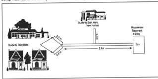
The 2.4-meters-long object represents the main underground sewer pipe. Place the cardboard box at one end of the "main sewer pipe," place two 0.6-meter-long objects to represent underground pipes coming from buildings where water is being used (homes, schools, restaurants, factories). Place the 0.7-meter-long object perpendicular to the middle of the "main sewer pipe." This object represents underground pipes coming from homes recently constructed in the community.
