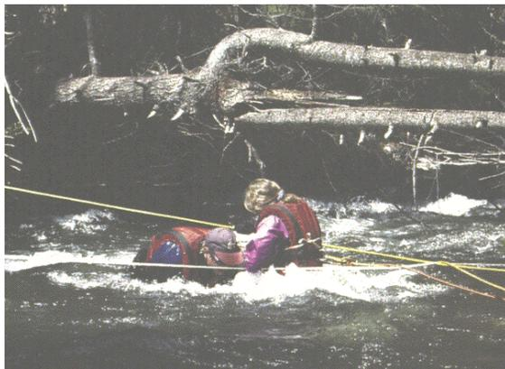
Fig. 4: Emptying Bedload Traps at Above Bankfull Flow at Cherry Cr., 1999.
