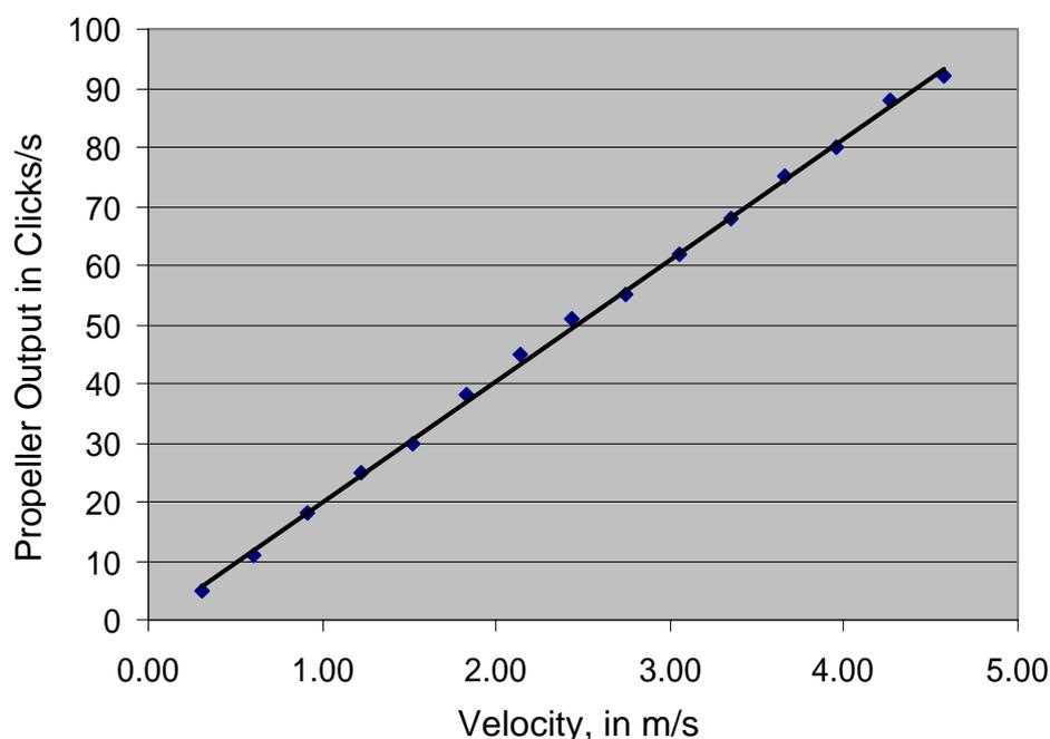
Fig. 4 LISST-SL tow-speed versus click rate of the propeller current sensor.
