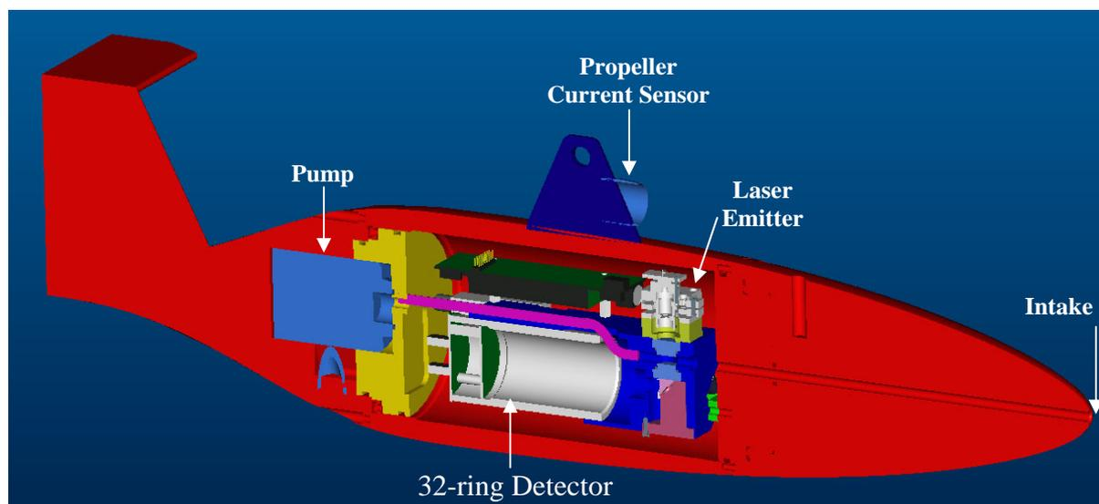
**Fig. 3** A cut-away view of the LISST-SL reveals the intake tube, laser source, ring- detector placement, and pump (this early drawing shows an upward-projecting tail fin; the LISST-SL tail fin now projects downward).
