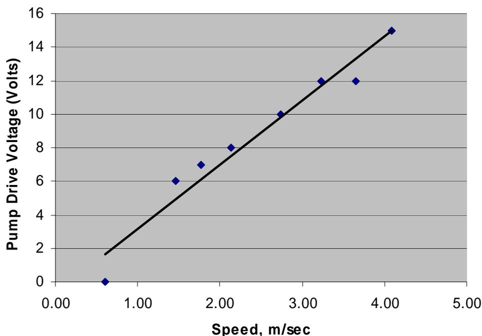
**Fig. 5** The relation between free-stream velocity and pump drive voltage. The relation includes consideration of the pressure head due to the flow. A perfect linear fit is not expected due to pump discharge characteristics.
