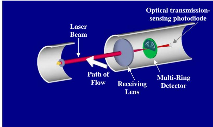
**Fig. 1** A cut-away of the optics shows a laser beam traveling left to right, a receiving lens, a multi-ring detector, and an optical transmission-sensing photodiode. Particles flow with water at the arrow.
