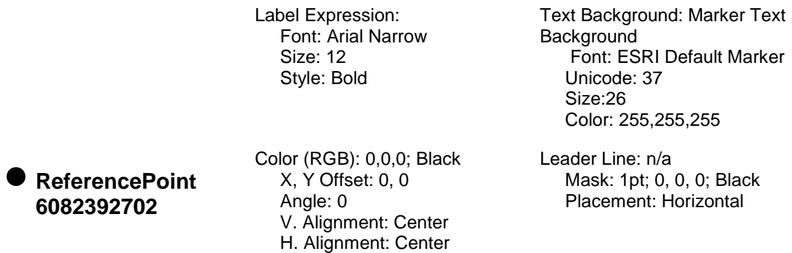
Figure 3.4. ReferencePoint Point Cartographic Standard
