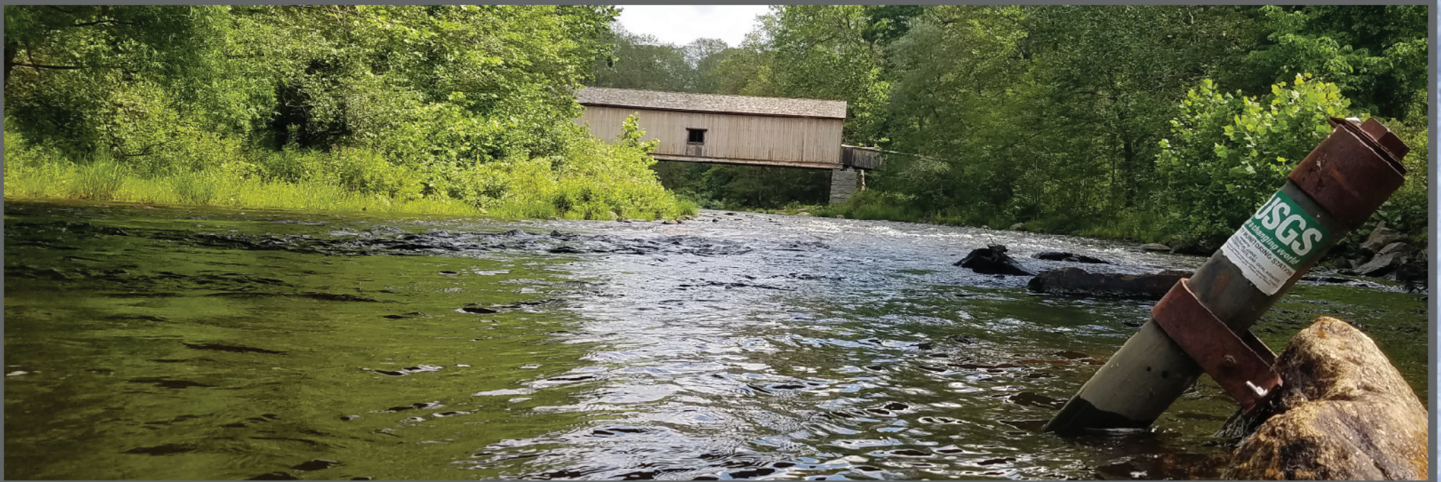
01193500 Salmon River near East Hampson, Connecticut, shows housing for water-quality monitor (YSI 6920) for Dissolved Oxygen Project, in cooperation with the Connecticut Department of Energy and Environmental Protection. Brittney Jones (photographer); May 2017.
