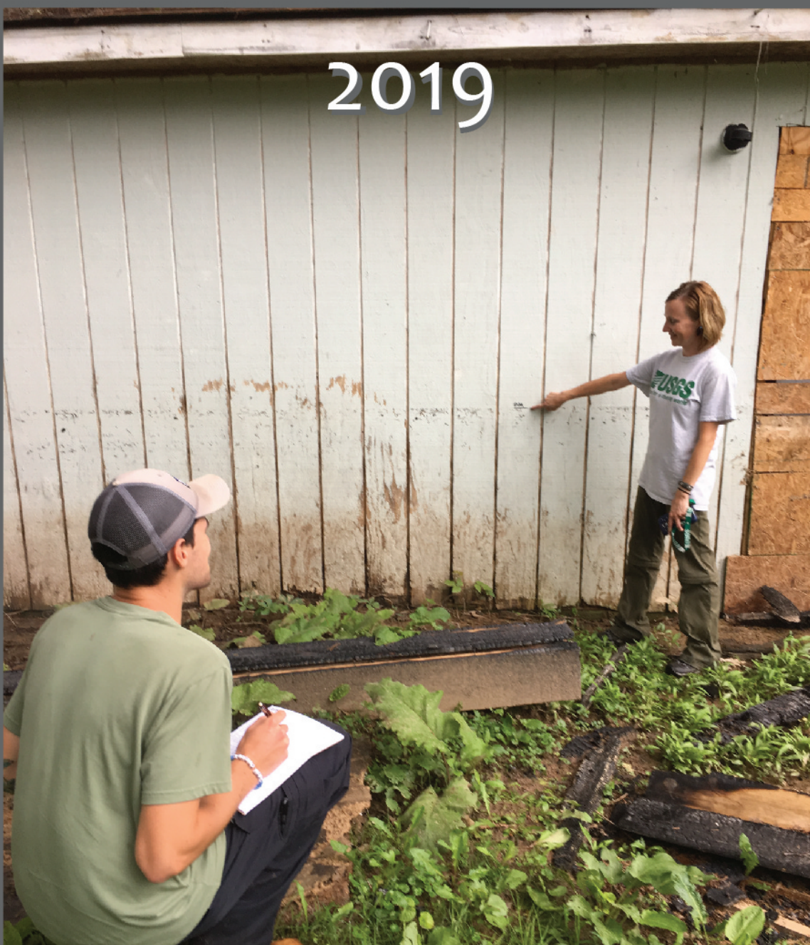
Identification, documentation, and flagging of high water marks in the town of Alderson, West Virginia, after the June 2016 floods. Shephan Shansey and Jerilyn Collenburg (New Jersey Water Science Center) pictured. Study done in cooperation with Federal Emergency Management Agency and the Virginia-West Virginia WSC, near 03183500 Greenbrier River at Alderson, West Virginia. Jim Duda (photographer); July 2016.
