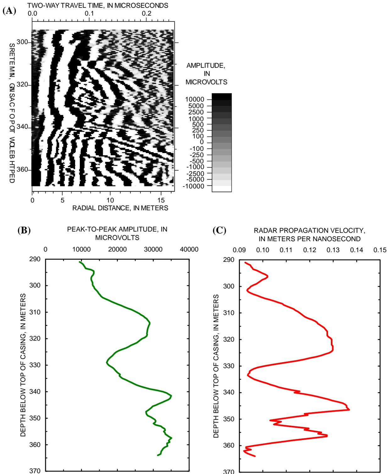
**Figure 6.** Radar reflection logging in borehole HC-2, Project Shoal Area, Churchill County, Nevada: (A) 60-megahertz electric-dipole omni-directional radar reflection log, (B) direct-wave amplitude log, (C) direct-wave radar velocity log.
