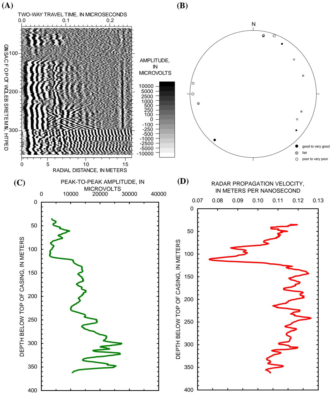
**Figure 9.** Radar reflection logging in borehole HC-7, Project Shoal Area, Churchill County, Nevada: (A) 60-megahertz magnetic-dipole directional radar reflection log, (B) lower hemisphere equal-area stereo-net showing poles of interpreted reflectors, (C) direct-wave amplitude log, (D) direct-wave radar velocity log.
