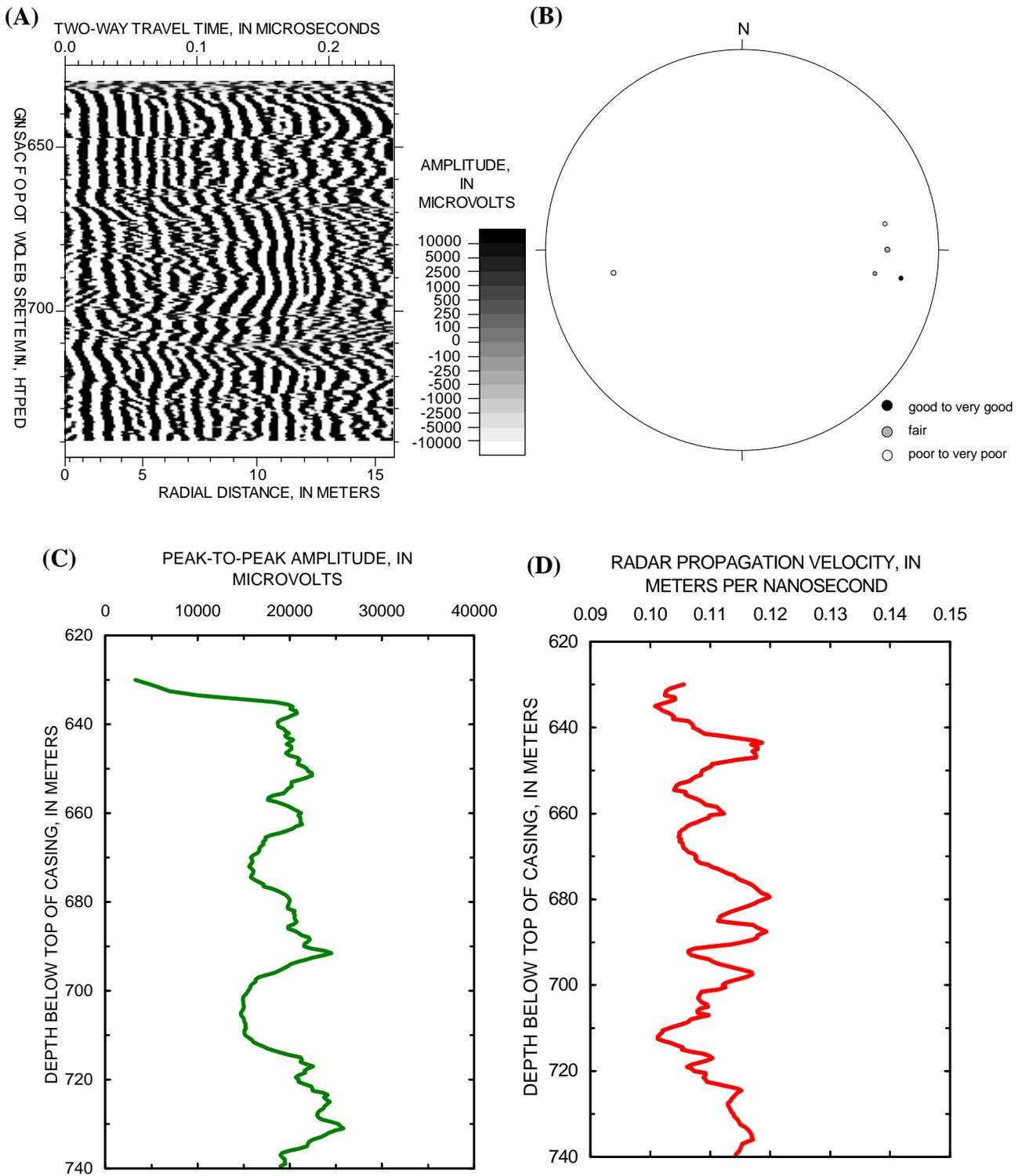
**Figure 10.** Radar reflection logging in borehole HC-8, Project Shoal Area, Churchill County, Nevada: (A) 60-megahertz magnetic-dipole directional radar reflection log, (B) lower hemisphere equal-area stereo-net showing poles of interpreted reflectors, (C) direct-wave amplitude log, (D) direct-wave radar velocity log.
