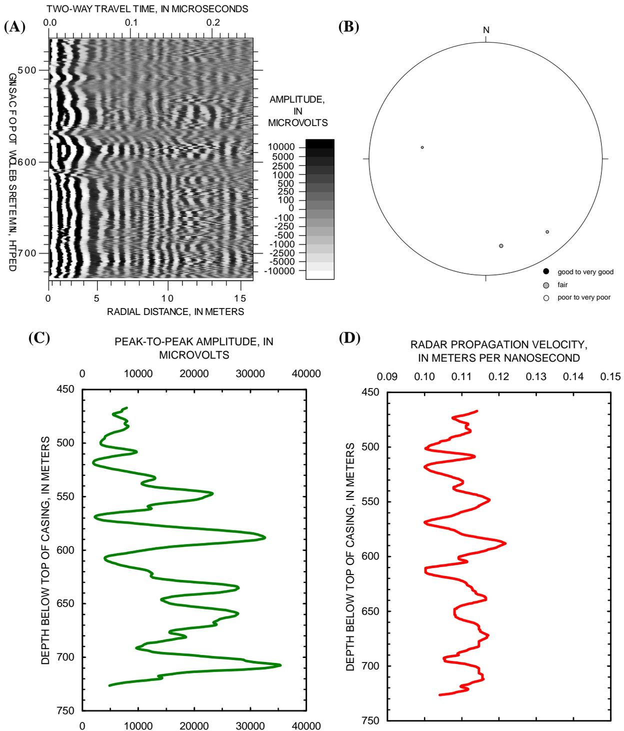
**Figure 7.** Radar reflection logging in borehole HC-5, Project Shoal Area, Churchill County, Nevada: (A) 60-megahertz magnetic-dipole directional radar reflection log, (B) lower hemisphere equal-area stereo-net showing poles of interpreted reflectors, (C) direct-wave amplitude log, (D) direct-wave radar velocity log.
