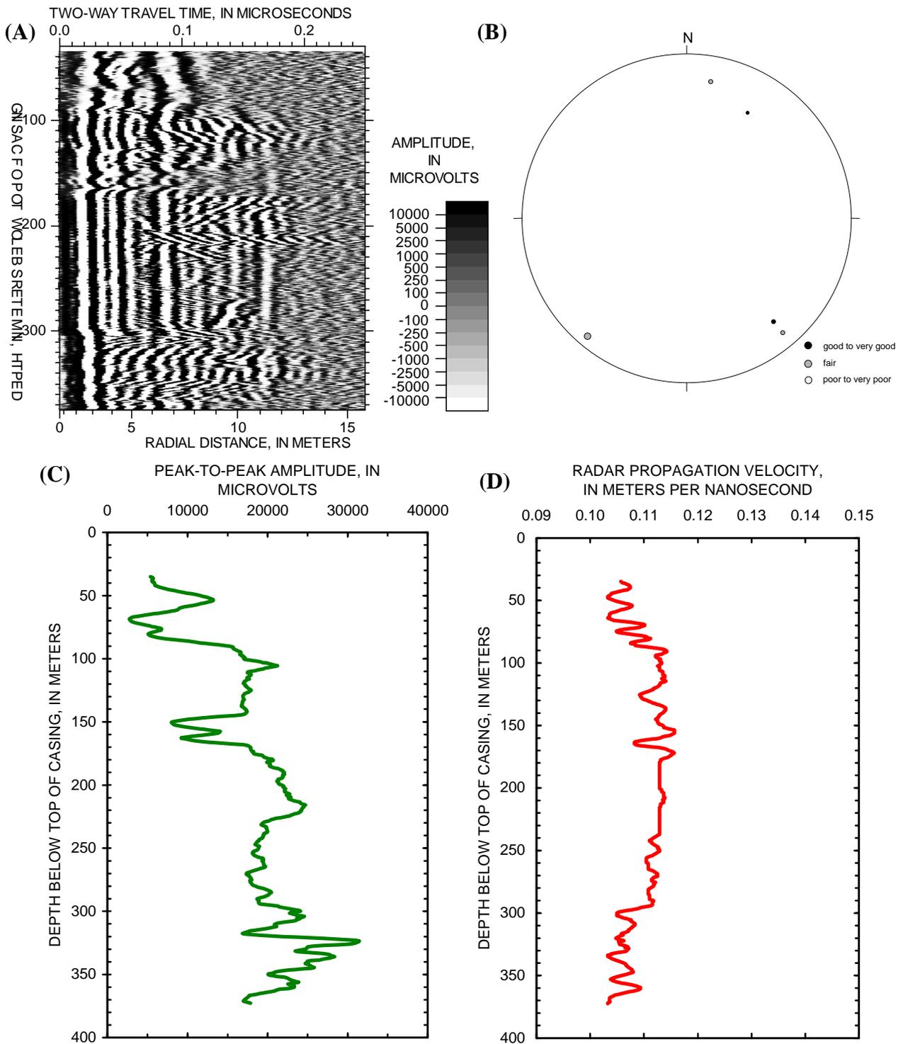
**Figure 8.** Radar reflection logging in borehole HC-6, Project Shoal Area, Churchill County, Nevada: (A) 60-megahertz magnetic-dipole directional radar reflection log, (B) lower hemisphere equal-area stereo-net showing poles of interpreted reflectors, (C) direct-wave amplitude log, (D) direct-wave radar velocity log.
