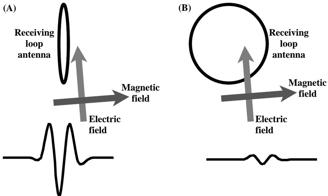
**Figure 3.** Effect of the orientation of a receiving loop antenna, with respect to an impinging transmitted electromagnetic wave, on the amplitude of the signal induced on the receiving antenna: (A) antenna loop parallel to incident electric field receives the maximum signal amplitude, (B) antenna loop perpendicular to incident electric field receives minimal signal amplitude.
