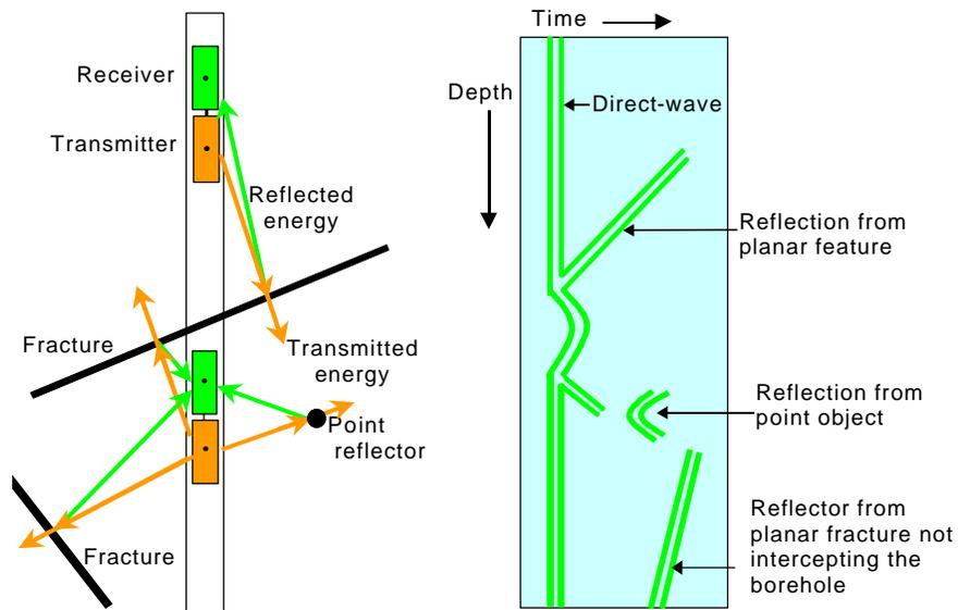
**Figure 2.** Transmitter and receiver antenna arrangement for borehole-radar reflection logging and the typical reflection patterns from planar and point reflectors.
