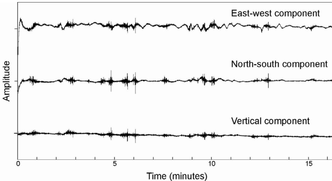
**Figure 5:** Representative 3-component ambient noise seismic records from Truro, Cape Cod, Massachusetts.
