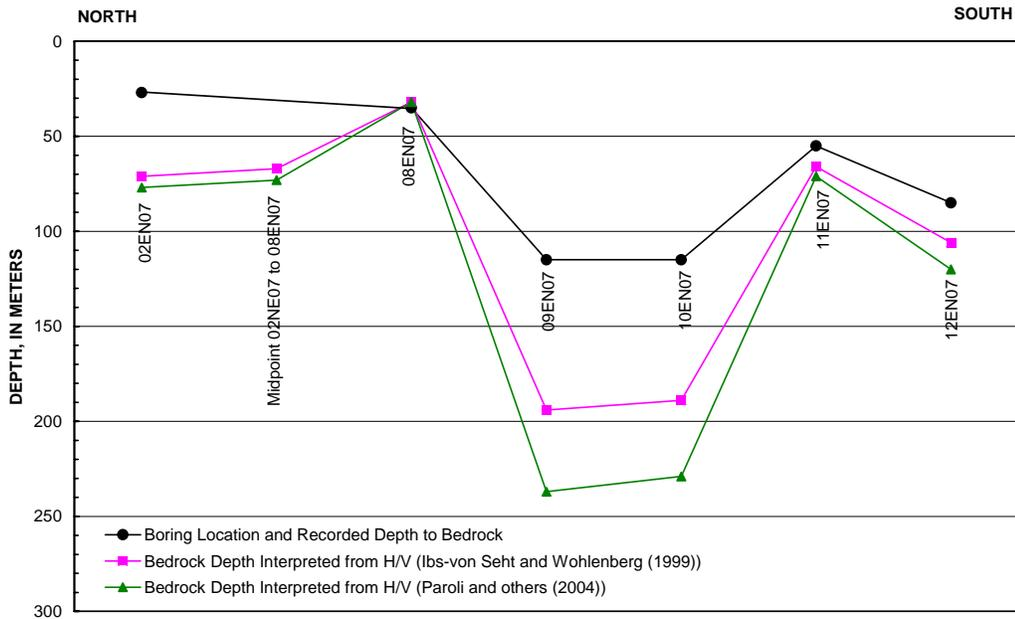
**Figure 9:** Profile of bedrock surface along transect near Firth, Nebraska, interpreted from H/V results, and depth to rock from adjacent boring logs.
