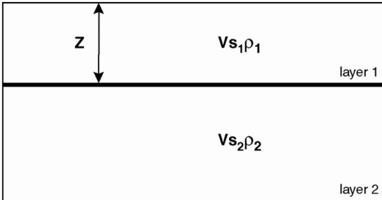
**Figure 1:** Conceptual earth model for H/V seismic method. The method assumes  $V_{s2}\rho_2 \geq 2V_{s1}\rho_1$ , where  $V_{s1}$  and  $V_{s2}$  are the shear wave velocities in layers 1 and 2, respectively, and  $\rho_1$  and  $\rho_2$  are the densities in layers 1 and 2, respectively.  $Z$  is the thickness of layer 1 (sediment).
