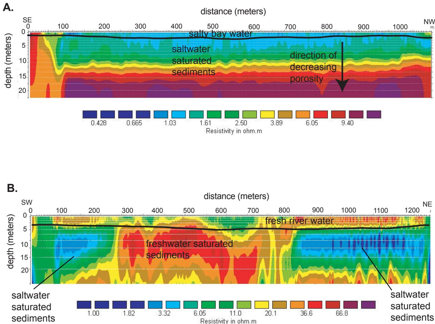
**Figure 2.** Inverted resistivity section WB18 with interpretations (A) and WB21 with interpretations (B). The inverted model displayed for WB18 is the third iteration with a root mean squared error (RMSE) of 3.3%. The inverted model displayed for WB21 is the fifth iteration with an RMSE of 4.3%. Water bottom measured by an echo sounder is plotted as a dark line.
