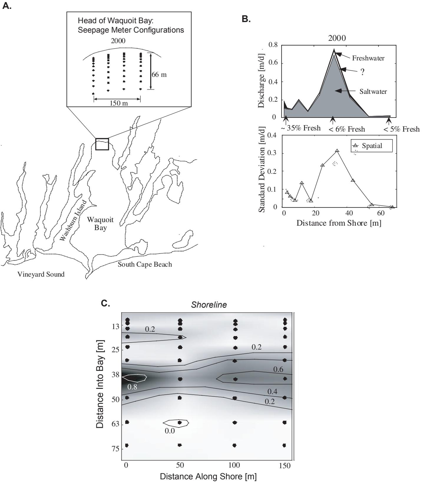
**Figure 5:** Results of seepage meter study in Waquoit Bay by Michael et al. (2002). Figure and data reprinted with permission. (A) Location of seepage meters (B) distribution of freshwater and saltwater in discharged water with distance from shore, and (C) time-averaged ground-water discharge in meters per day.
