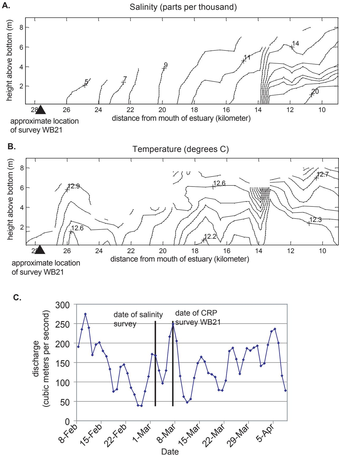
**Figure 3.** Salinity (A) and temperature (B) profiles of Winyah Bay on March 3, 2002. Average daily stream flow (C), Pee Dee River USGS Gaging Station 02131000 (at Peedee, South Carolina).
