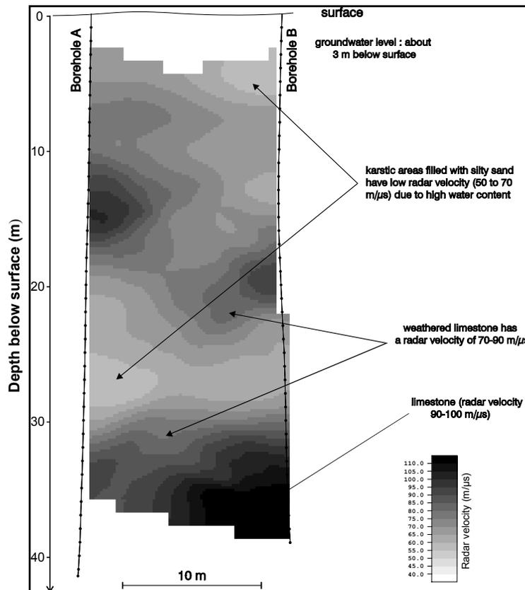
**Figure 4.** Borehole radar velocity tomogram showing karstic features in limestone (from Corin et al., 1997). [m/μs is meter per microsecond.]
