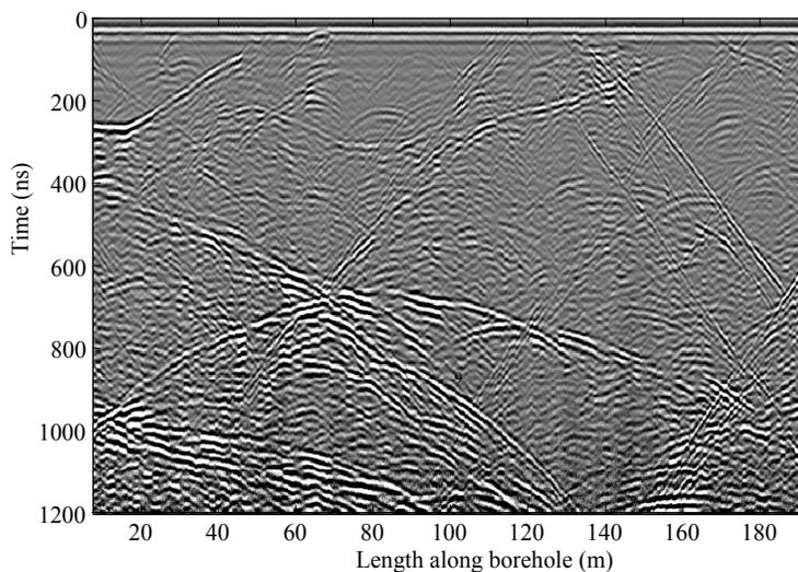
**Figure 2.** Borehole radar in an inclined borehole, using 100 MHz antennas. The reflectors are due to thin dykes and to fractures.
