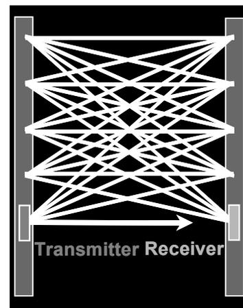
**Figure 3.** Ray coverage of cross-hole tomography.
