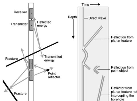
**Figure 1.** Orientation of transmitter and receiver in a single borehole and the resultant radar record from a fracture and a point reflector
