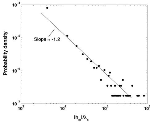
**Figure 2.** Spectrum of hydraulic head in Sugar Creek using 784 terms in the Fourier series. The frequency decays with increasing amplitude-to-wavelength ratio,  $|h_m|/\lambda_x$ . Essentially, the data set does not contain enough points to provide a statistically high-quality representation of the infrequent features contained in the tail of the topographic distribution.
