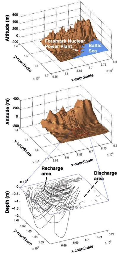
**Figure 1.** (top) Map data from the Swedish National Land Survey covering an area of 40,000 km<sup>2</sup> (middle) with the National coordinate system RT 90 compared with Fourier surface using 784 terms. Higher resolution around the central area marked with a red rectangle gives higher weight of this area when the Fourier coefficients are determined. (bottom) Flow trajectories with dis- and recharge areas with assumption of groundwater flow extending to a depth of 20 km in the crust.
