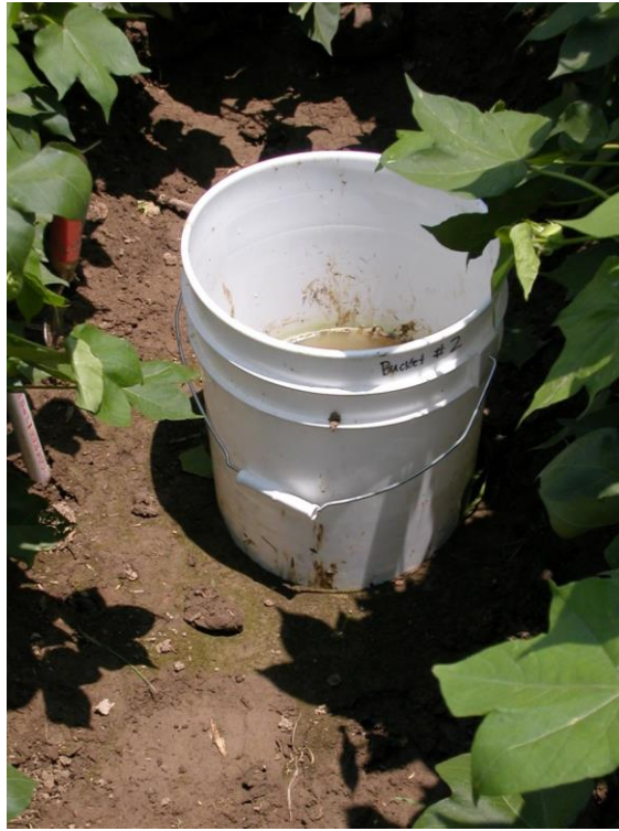
Figure 19. Bottomless bucket method setup for a location in the Mojave Desert, USA. The photograph illustrates the simple equipment (a bucket with the bottom cut out), stopwatch, and ruler (not shown) to measure the declining water level in the bucket. These values are used to estimate the surface permeability of the unit. These values, in turn, can be used to estimate recharge.
