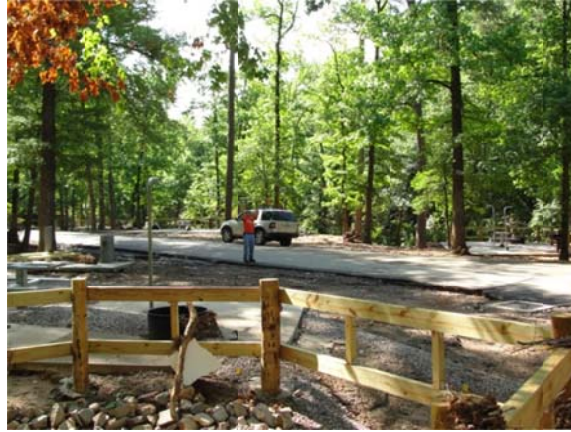
Looking from upstream diagonally to the XS2. Note location of high water marks as shown by hydrographer holding rod horizontally.
