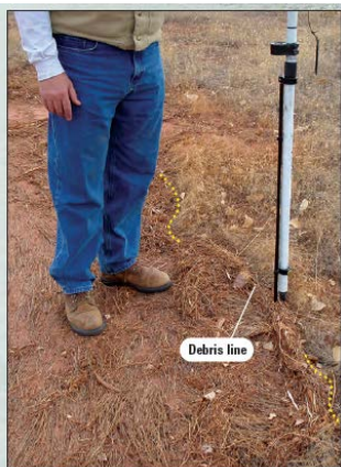
Figure 12. A hydrographer surveying the landward edge of a debris line. Photograph by Christopher Wilkowske.
