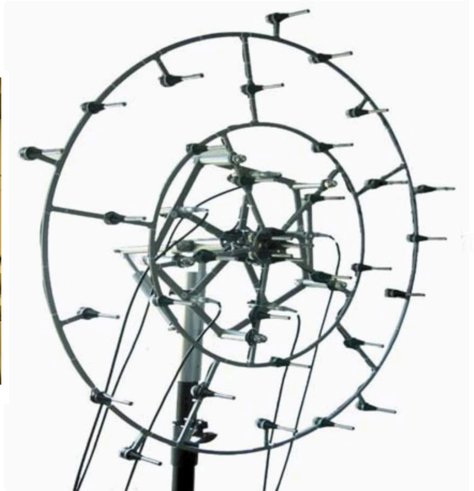
117-element Phased Array installed in the VT anechoic wind tunnel
