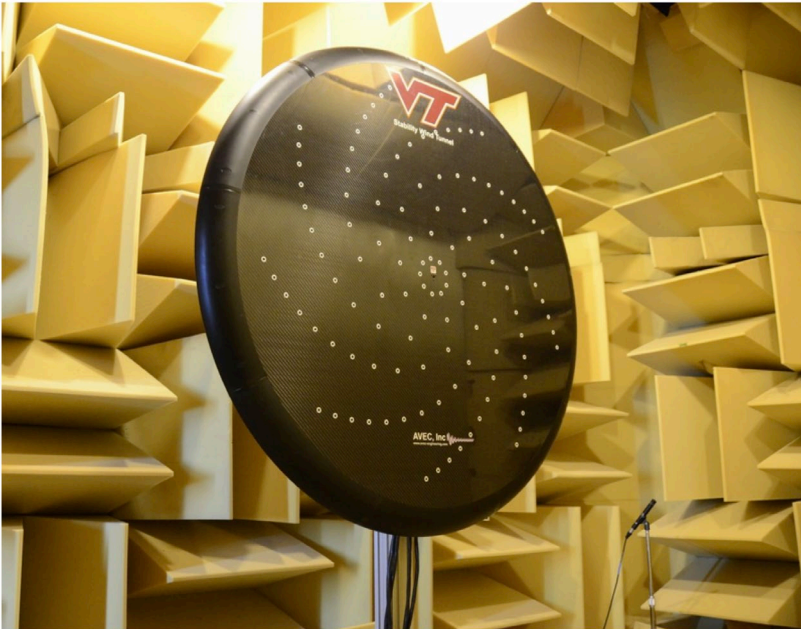
117-element Phased Array installed in the VT anechoic wind tunnel
