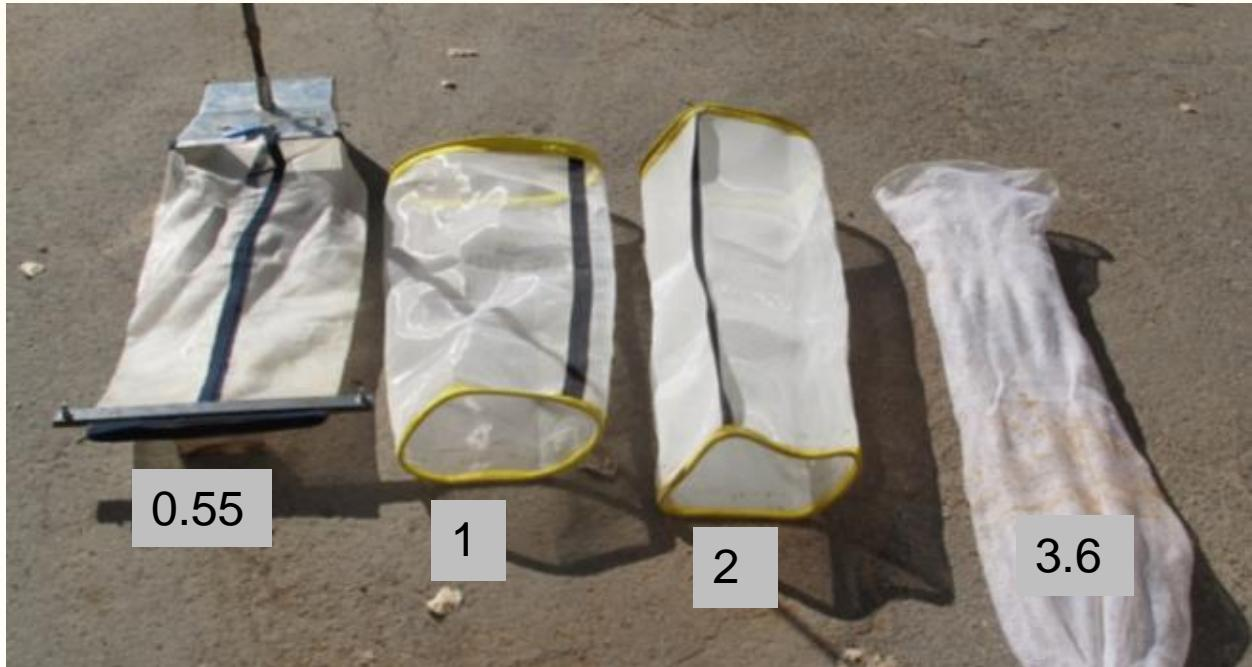
Nets with various mesh width (mm) tested for TR2 sampler
