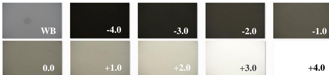
Figure 3 Typical 10-frame dataset showing white balance reference card (WB) and -4 to +4 exposure value (EV) bracketing sequence. This example was acquired during diffuse (overcast) ambient lighting conditions.
