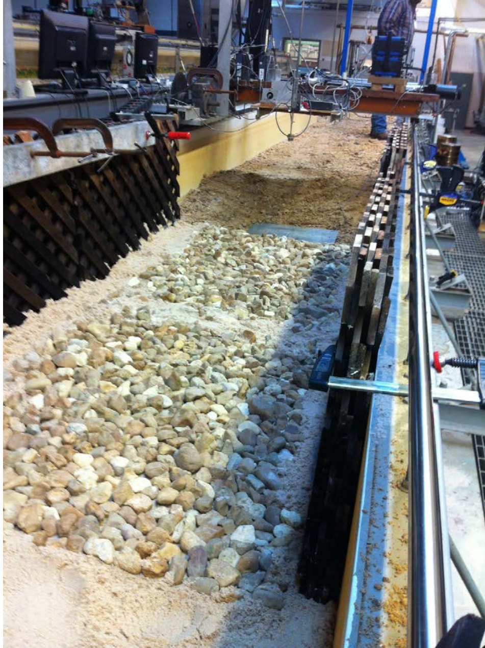
Figure 2. The flume test-section configured for the rock-towing experiments. Gravel substrate shown has been rigidly fixed to an underlying plywood bottom set atop a layer of sand. Individual particles (Table 1) were then towed across the substrate using the instrument cart above the flume in the photo.
