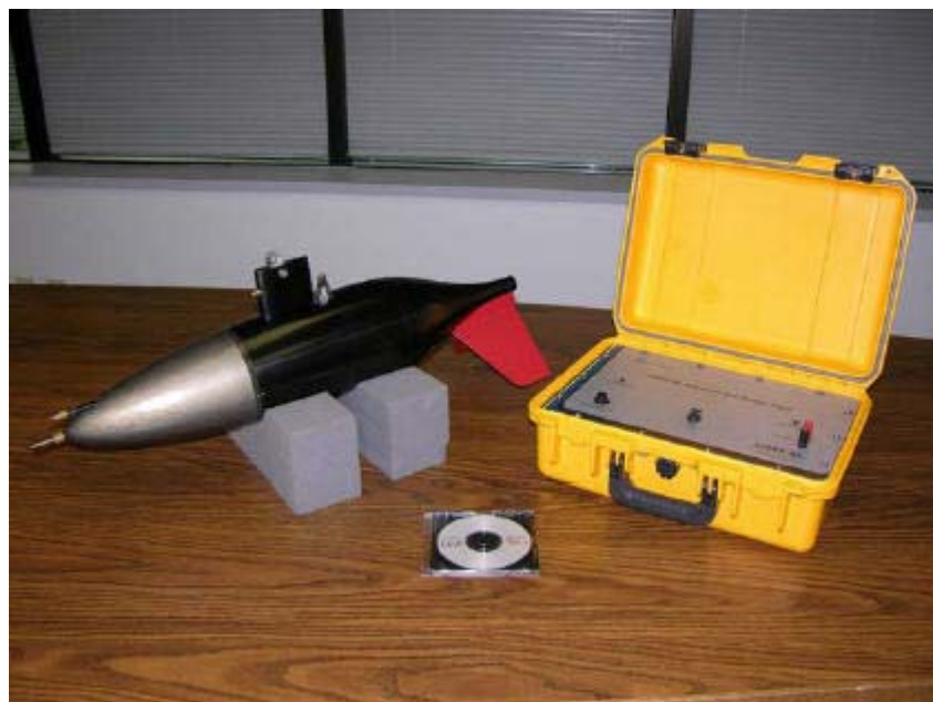
Figure 1-- The LISST-SL and Topside Control Box
