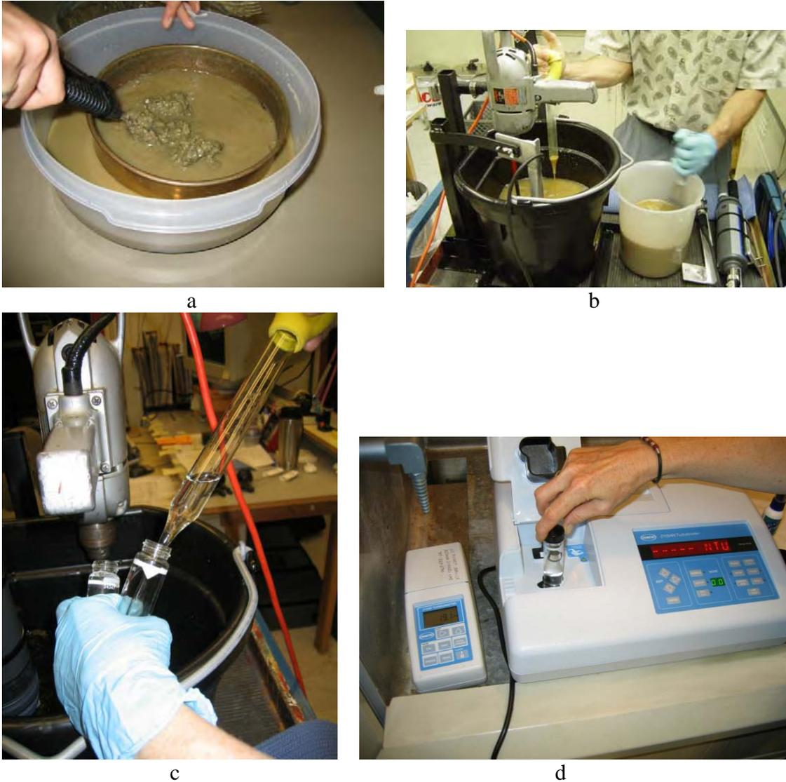
**Figure 5.** (a) wet-sieving to 0.5 mm, (b) adding sediment from the slurry to the mixing bucket, (c) subsampling from the mixing bucket for (d) Hach measurements.
