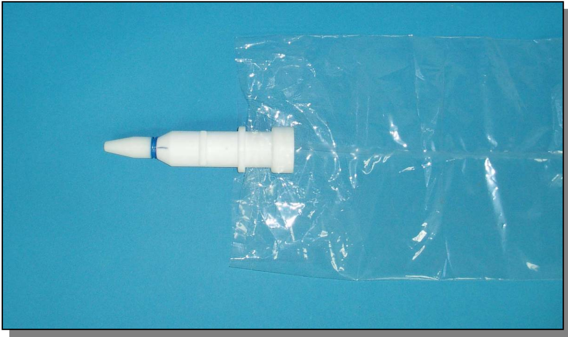
Figure 12-- Nozzle holder placed in center of bag opening
