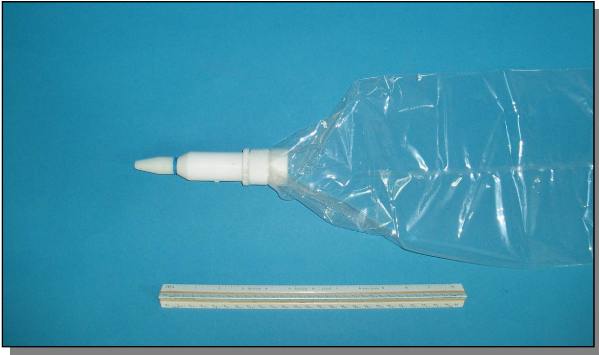
Figure 6-- Nozzle holder with nozzle and bag attached
