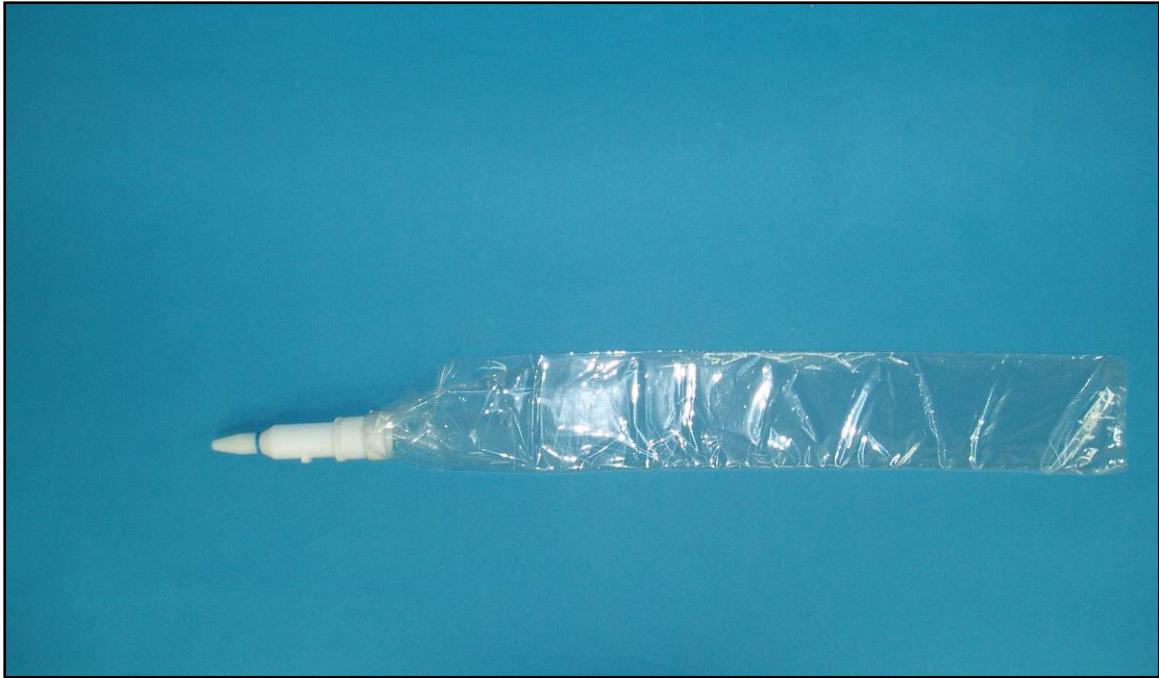
Figure 14-- Bag folded and pressed to remove air
