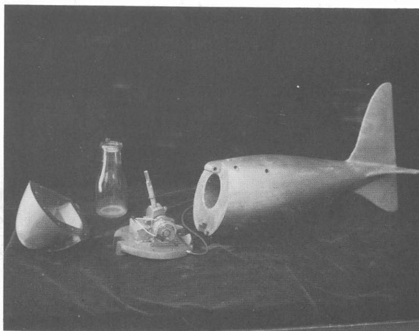
Fig. 10 Point-integrating suspended-sediment sampler, US P-46, head cover and head base removed
