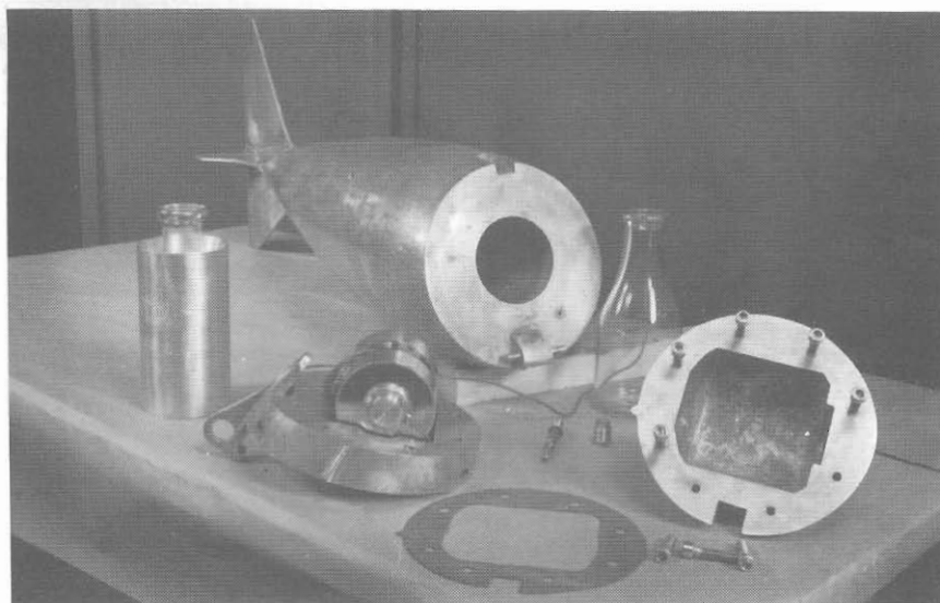
Fig. 15 Point-integrating suspended-sediment sampler, US P-50, head cover and head base removed
