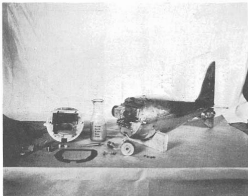
Fig. 45b--Valve mechanism for P-46 E sampler, disassembled
