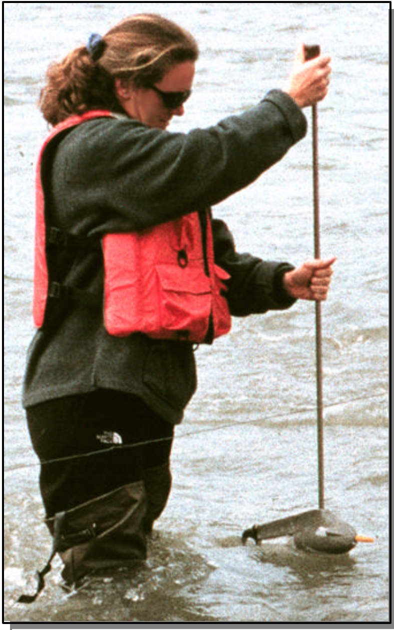
Figure 4. Proper wading sampling stance using a US DH-48 sampler
