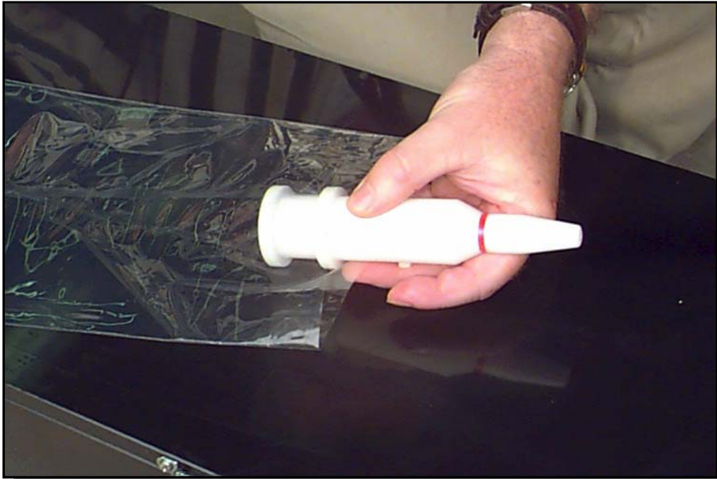
Figure 5-- Place nozzle holder in center of bag
