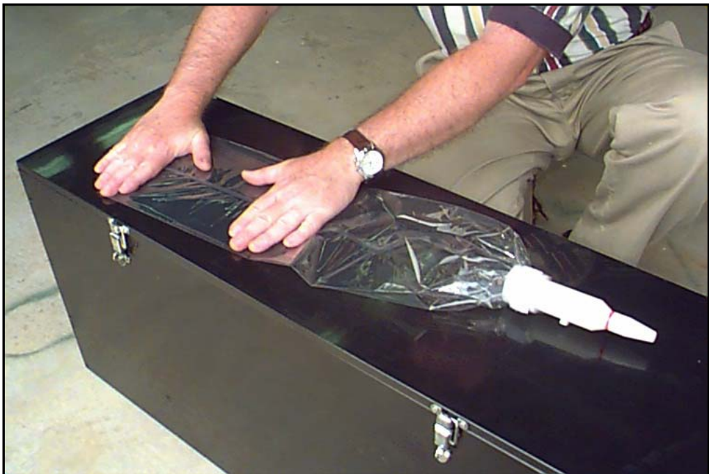
Figure 8-- Push air out of bag through nozzle
