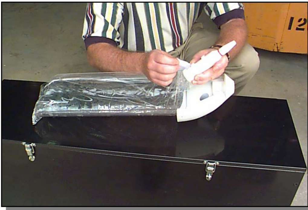
Figure 14-- Remove hook-and-loop strap
