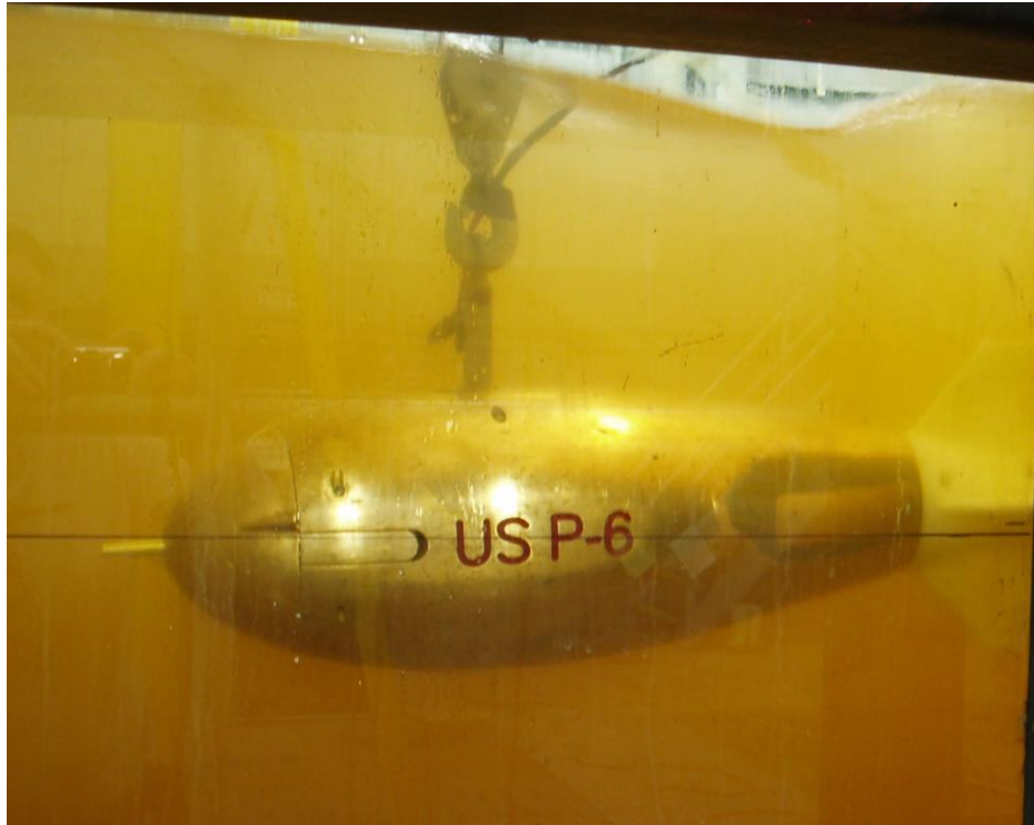
Figure 5—Photograph of tow-tank testing of P-6 sampler
