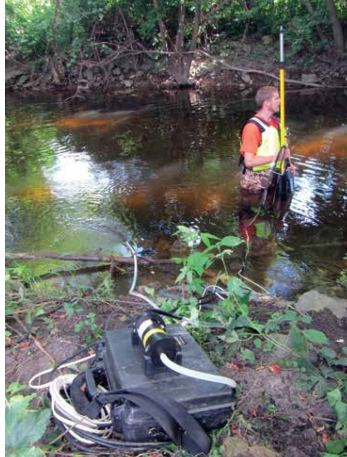
Figure 6. Field testing a custom in situ fluorometer for detecting wastewater effluent near Madison, Wisconsin. Photo: Steve Corsi, USGS.
