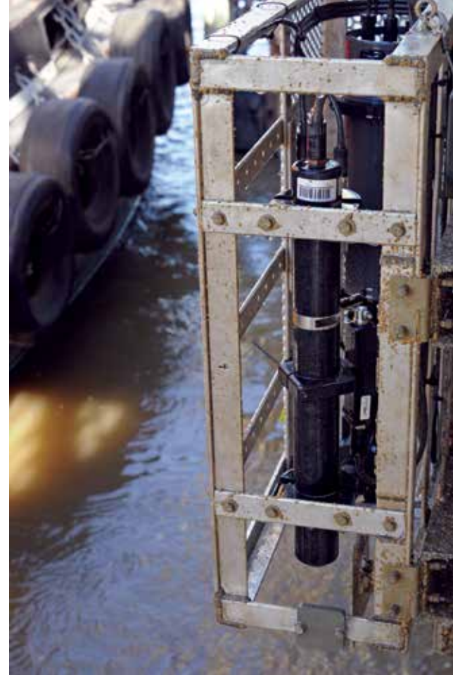
Figure 2. Continuous UV nitrate sensors and other water-quality instruments deployed in the Mississippi River at Baton Rouge (USGS gage 07374000) allows for a better understanding of nitrogen dynamics at the rates in which changes occur.
